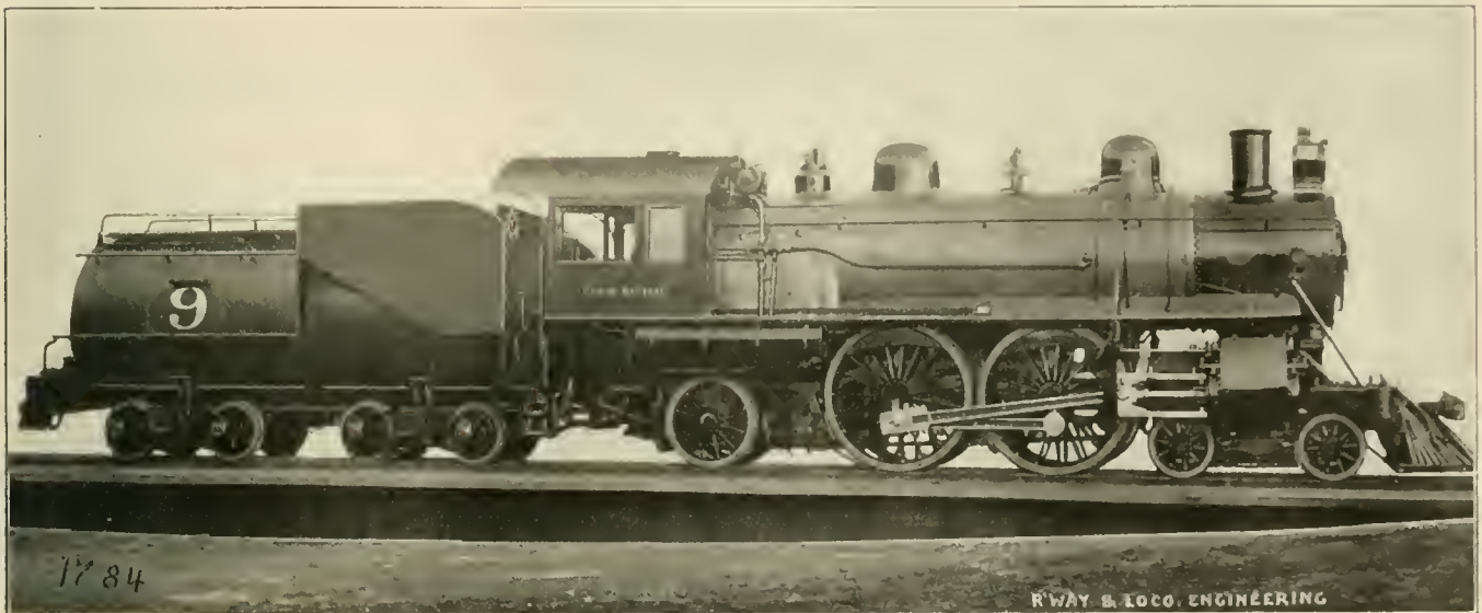
ATLANTIC TYPE PASSENGER ENGINE, WITH VANDERBILT TANK, FOR THE UNION PACIFIC.
